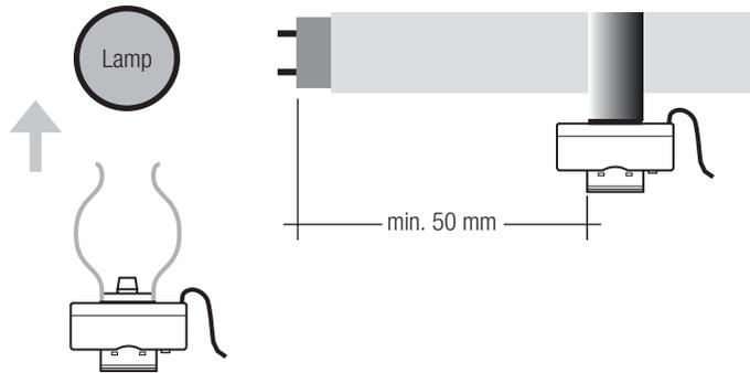
**Mounting with cover frame in luminair housing:**
