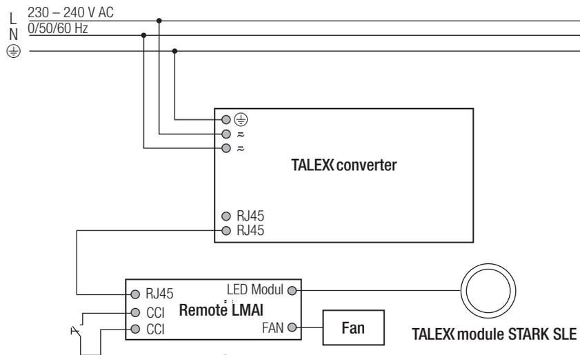
Operating with continuously variable potentiometer
