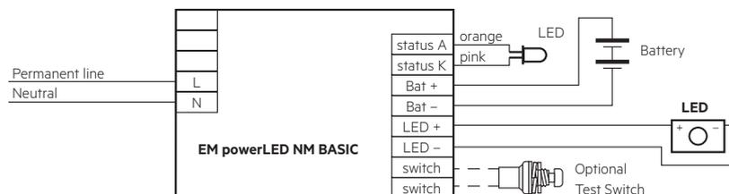
Take care that the LED is connected with the right polarity. LED that are connected to the EM powerLED devices should have a reverse polarity protection device such as a schottky diodes fitted, otherwise irreversible damage could occur if the LED is connected in reverse polarity. Any protection device must be capable of handling in excess of 700 mA.
