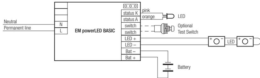
Wiring diagram for multiple LED (3–12) in parallel
