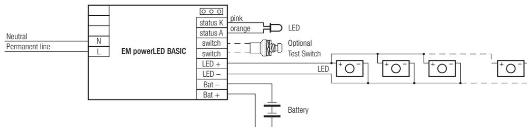
Take care that the LED is connected with the right polarity. LED that are connected to the EM powerLED devices should have a reverse polarity protection device such as a schottky diodes fitted, otherwise irreversible damage could occur if the LED is connected in reverse polarity. Any protection device must be capable of handling in excess of 1,000 mA.
