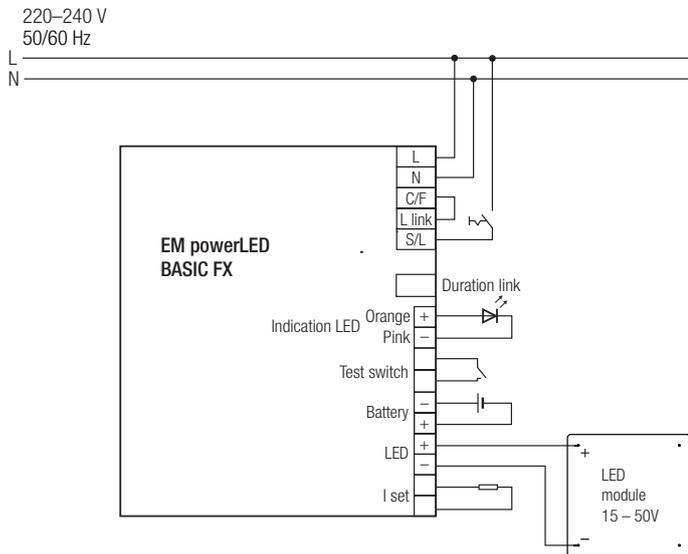
Wiring diagram EM powerLED BASIC FX with sensor
