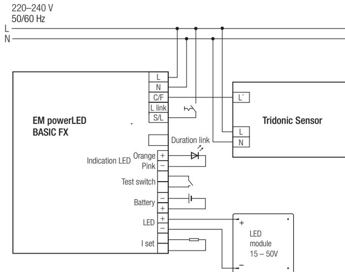
When using the EM powerLED without a sensor, connect the terminals C / F and L link with a wire.
