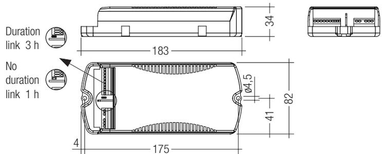
Note: LED Driver supplied with duration link in 3 hours position. Remove duration link for 1 hour duration. Duration link and I-SELECT PLUG must be set before battery and mains connection.
