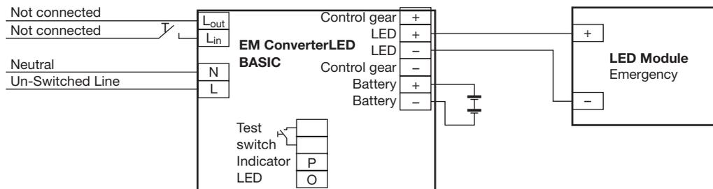
**EM converterLED BASIC with a standard LED Driver and one LED module for mains and emergency operation**
