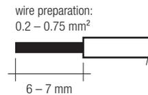
Inserting stranded wires / removing wires by lightly pressing on the push button.
