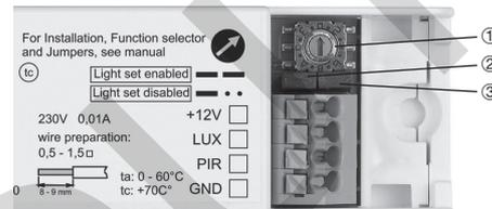
① Rotary switch operation mode
