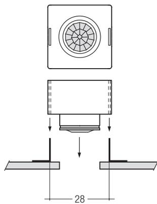
With long mounting clamps the sensor can be adjusted up or down so the sensor edge is flush with the surface of the luminaire.
