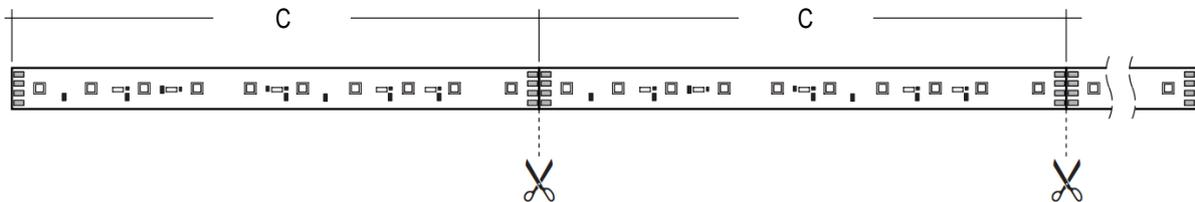
When cutting the IP65-version it is recommended to use the included silicon kit to re-seal the LED-tape according to the instructions on page 5.
