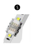
Repeat steps 1-4 for the other connecting end of the LEDtape. Make sure you check that both ends are facing the SAME POLARITY before locking the last connector in place.
